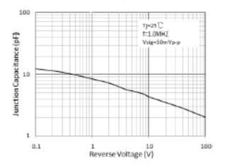
Figure 4. Typical Junction Capacitance
